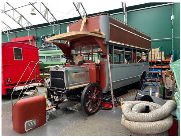
Meanwhile there is excellent progress on T448. The interior is ready to receive the seat frames and the engine overhaul is progressing well.
