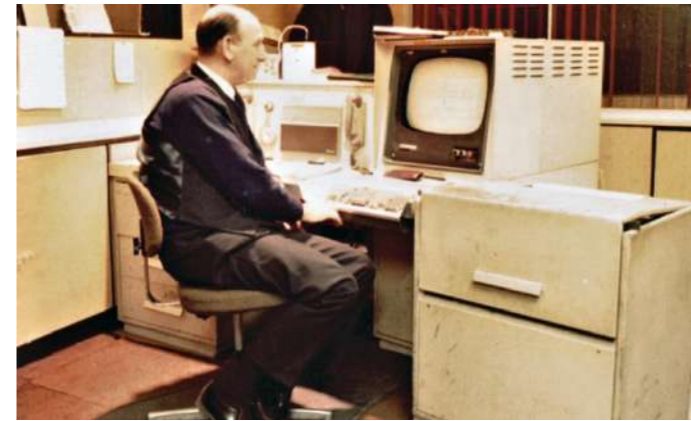
A route controller sits in front of a CARLA installation. That equipment, introduced by LT in 1979, was a system which included a two-way bus radio links. Those had initially been provided to combat rising staff assault rates. The system, headquartered in the Mansion House, was uprated to provide a network linking inspectors in radio equipped cars and emergency response vehicle crews, allowing those to respond to problems reported by on-route bus drivers. The computer screen showed the location of individual buses and the schedules which they were operating. That provided the CARLA operator with the information needed to direct actions to improve service levels, particularly on trunk routes, such as Mortlake's no 9.
